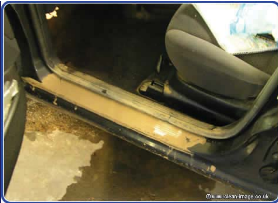
Silt on door shuts.
