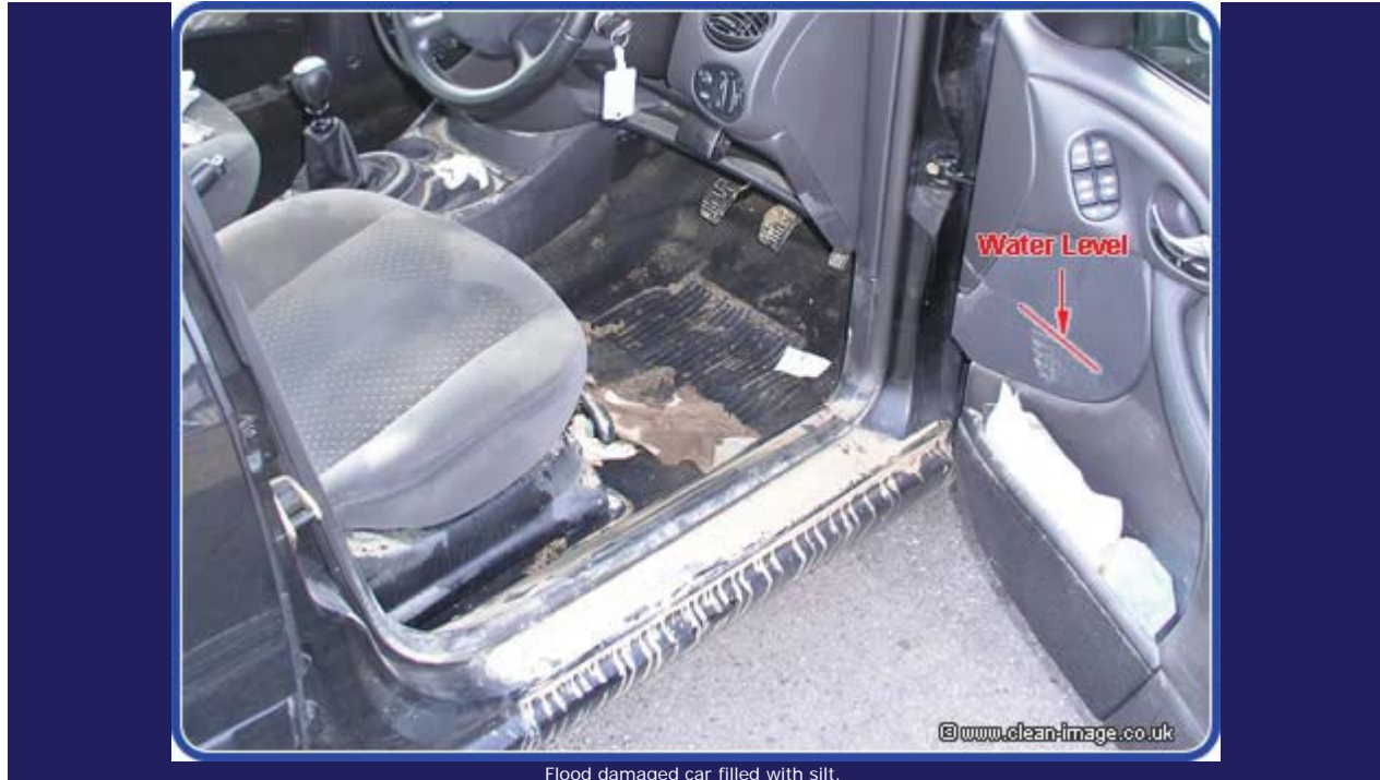
Flood damaged car filled with silt.
