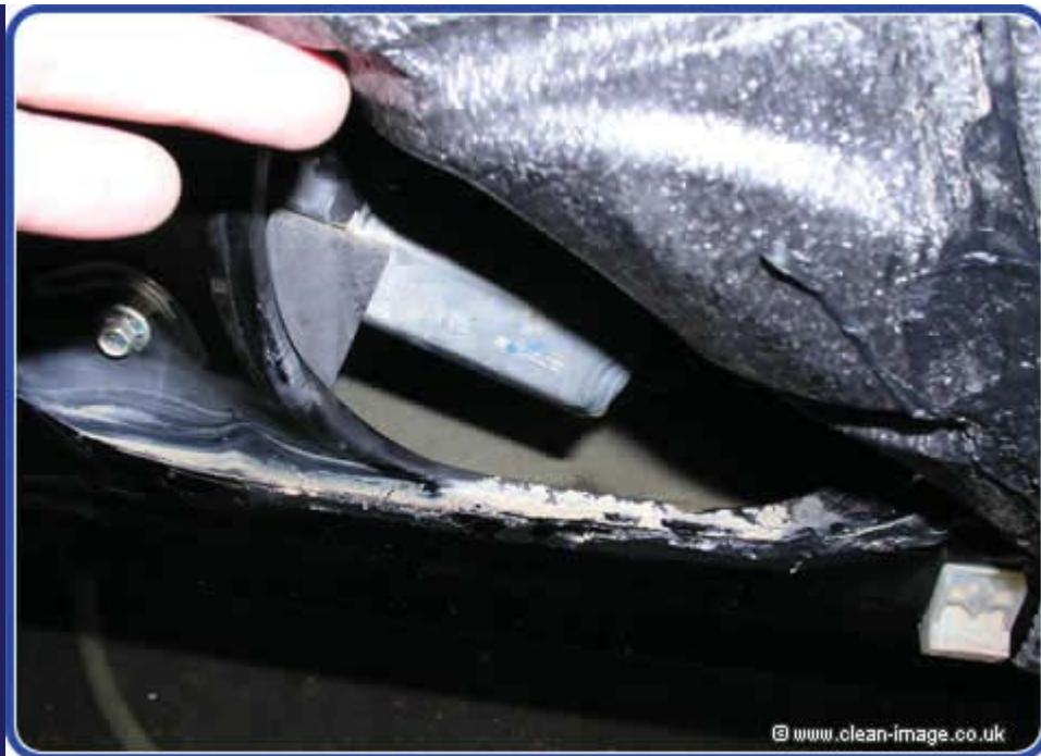
Silt and sediment from the flood behind the door skin.
