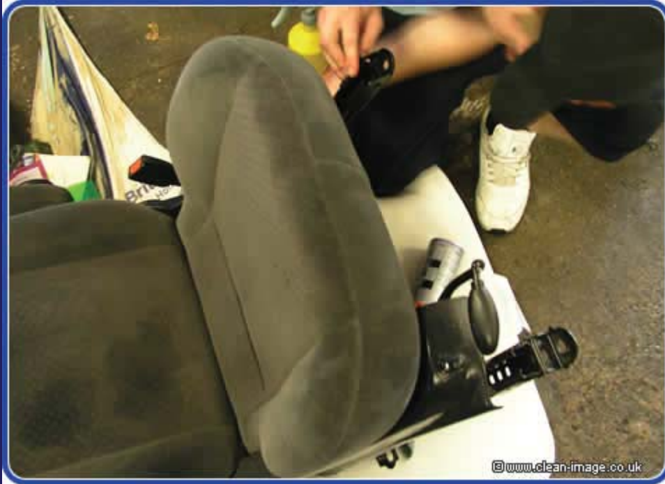
Detailing and lubricating the underside of the seats.
