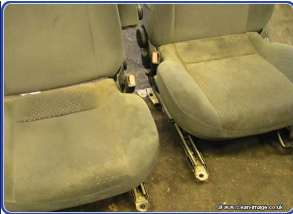
Flood damaged seats filled with silt.
