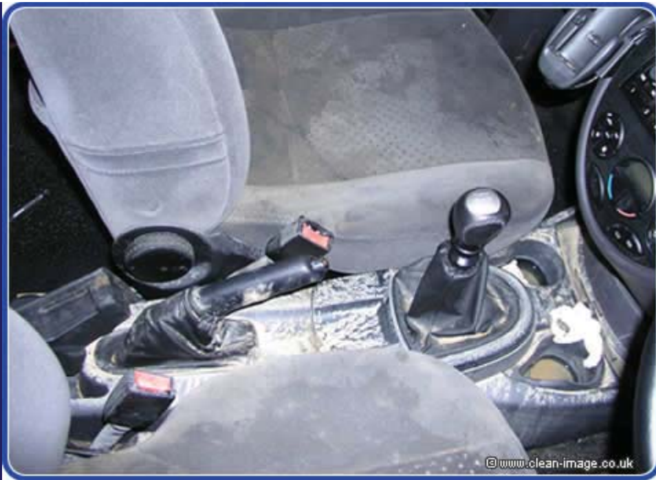
Centre consul covered in silt. Water still in the cup holders.
