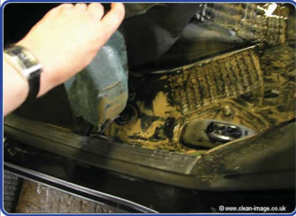
Silt from clay has penetrated through the carpets.
