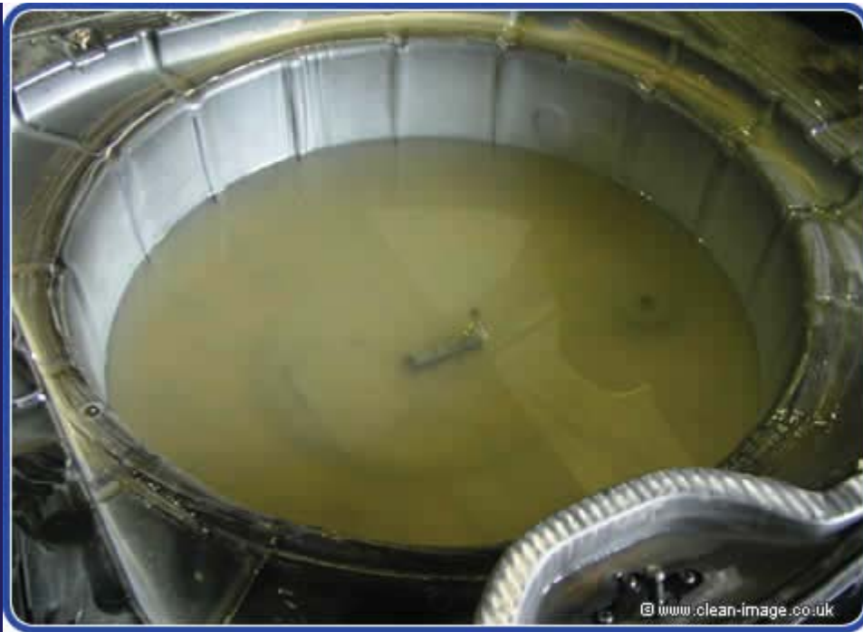
Flood water in the spare wheel area.
