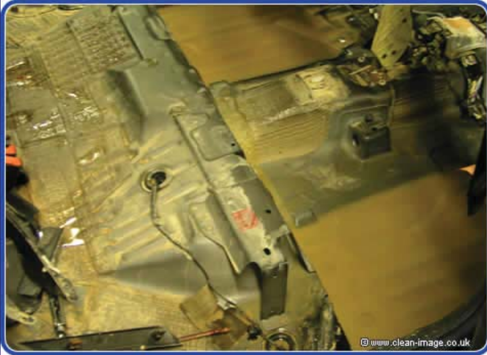
Flooded footwells, with the carpet removed you can see the amount of water and silt still in the car.
