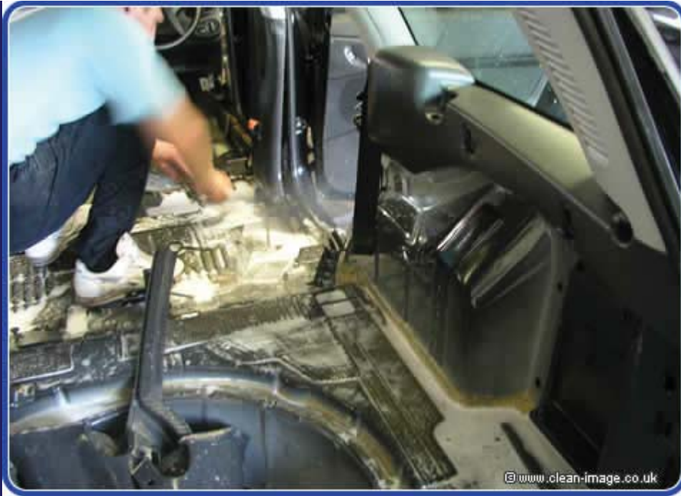
Panels and trim are removed.
