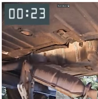
Removing a catalytic converter with a portable shear in 23 seconds
