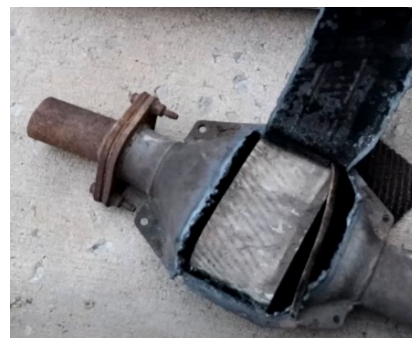
Cutting open a detached converter to remove the PGM coated honeycomb
